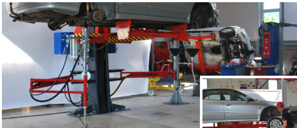
Drainage with TankDrillingMachine on swing arm
