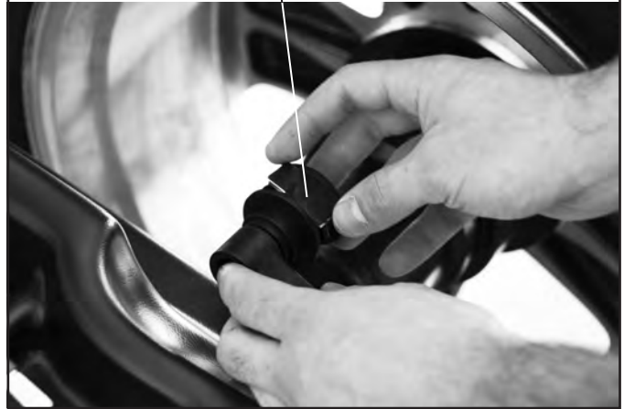
Fig. 49 Fit the adhesive weight in the pliers of the gauge rod
